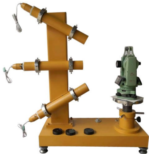
Collimator for auto level, theodolite, total station F4203T
